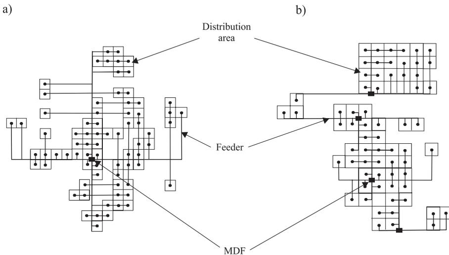
**Fig. 3. Calculation of ULL-costs with WIK-model: a) existing network (no clustering); b) optimised network (minimal spanning tree)**
