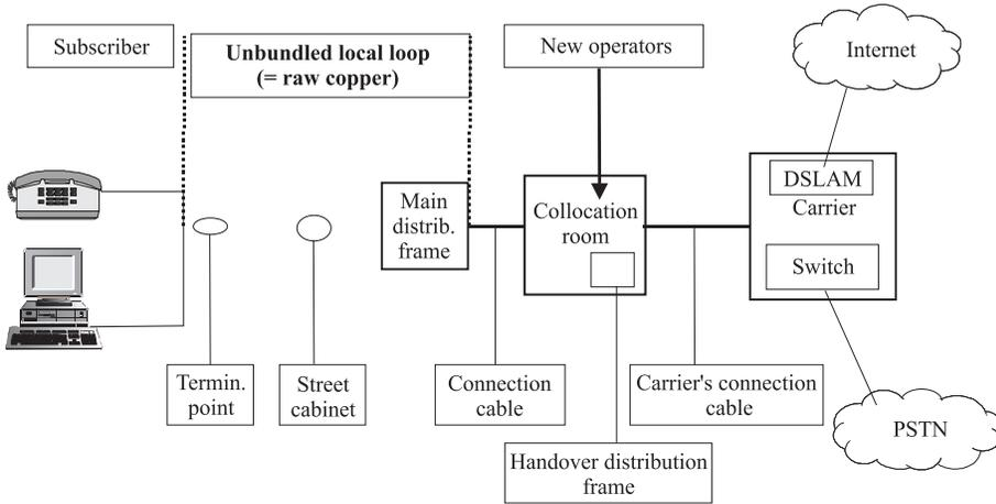
Fig. 1. Technical implementation of ULL access in Germany
