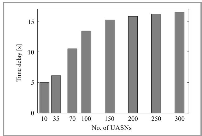
**Fig. 9.** Average time delay for different network sizes.
